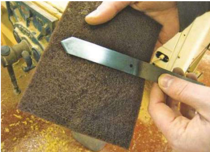
▲ Pic 8 The process left the metal black, which Dom rubbed off using a Hermes Webrax pad
